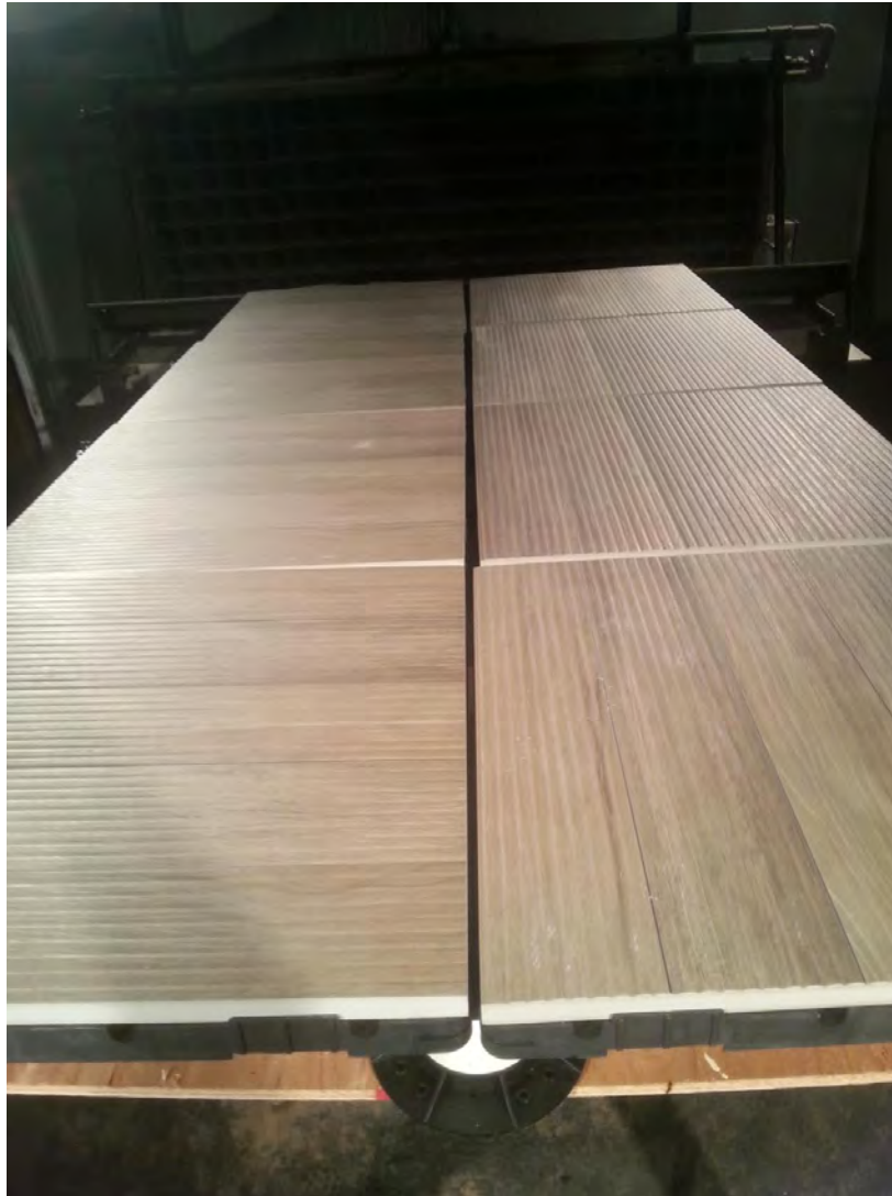
Photograph 1: Tile Tech Porcelain Paver Deck on Hex Tray Prior to Testing
